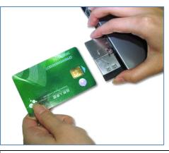
7. Smart card inserted in accordance with the direction of the arrow
